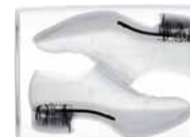
Inspecting for nail defects in shoes
