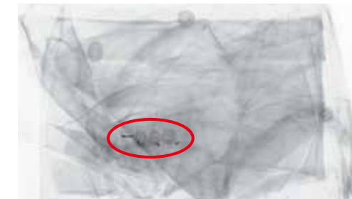
Broken sewing needle overlapping on clothes button in product
